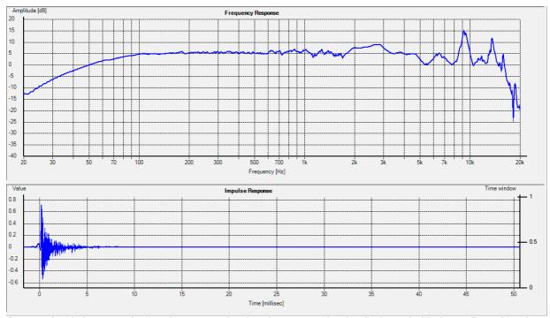
As can clearly be seen the low frequency rise has been completely eliminated, this is confirmed by the lower time trace which now tails off very rapidly, indicating at least theoretically that we can use this technique to measure accurately to very low frequencies.
