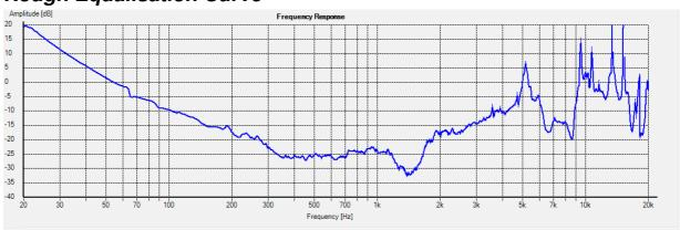
The resulting correction curve is reasonably clean at low frequencies but it is showing a considerable 45dB rise at low frequencies, however it is clearly completely inaccurate at high frequencies.
