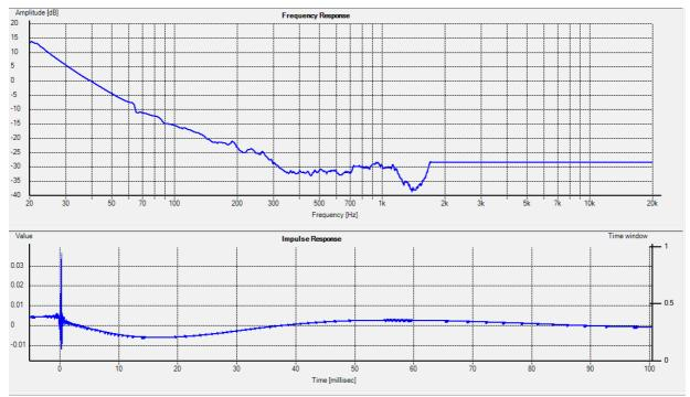
This then becomes the final correction or equalisation curve this can be directly applied to the Internal SPL curve either as a part of a Microphone or other correction or as a post process.
