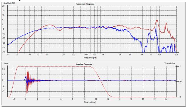
Measurements on a SEAS H1207 bass/mid driver; comparison between an IEC baffle as a ground plane Using TTC750 and TTC350 Tetrahedral Test Chambers.
