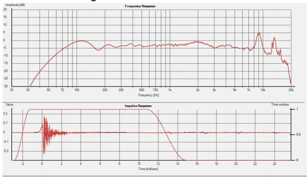
This clearly removes the majority of the reflection artefacts especially above 500Hz, where this result can justifiably be considered as anechoic. In theory a 12mS Window should be reasonably accurate below 160Hz and is often considered as safe down to 80Hz!
