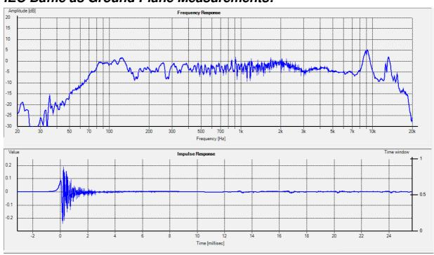
As can clearly be seen there are significant reflections however these mainly start after 10 to 12mS, the major impulse reflection starting at around 13mS the low frequencies being unreliable.
