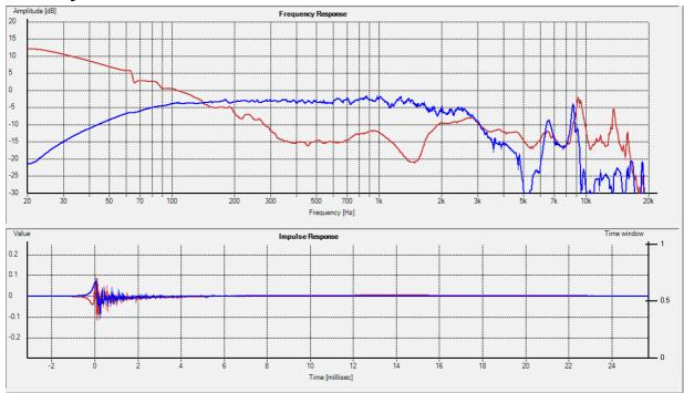
We will simply take the difference between these two curves the exact details differ between various measurement systems. This can be simply achieved in a spreadsheet by dividing these two curves. In practice this means subtracting the dB levels at each frequency in turn. Note Phase is NOT required.
