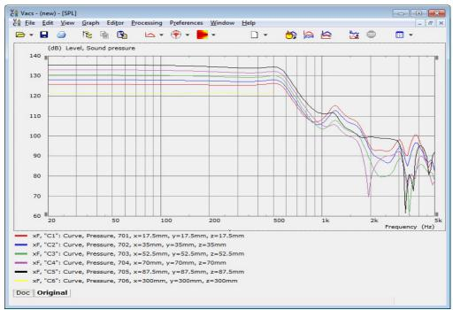
This clearly shows that below 500Hz the system works as a Pressure Environment, above this frequency there are some modes, which are effectively controlled by the Acoustic Absorption
