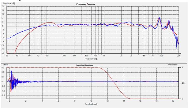
Clearly the low frequency response is accurate however the high frequency performance is also quite reasonably reliable within 5dB of the windowed response even without further correction which could be applied if higher accuracy were to be desired
